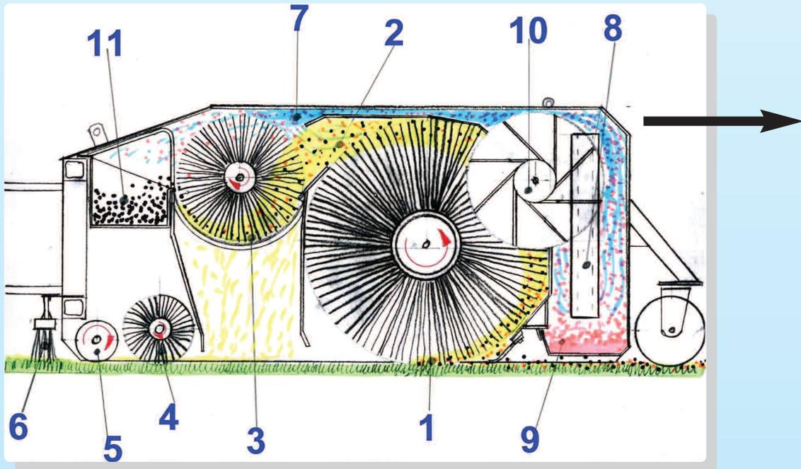
1. The soiled filling, sand, rubber granules or a mixture of both is picked up from the turf pile by means of a rotating brush.
